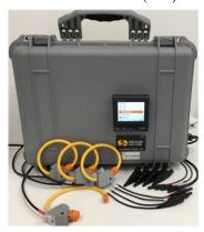
In addition to logging a range of power quality and energy parameters, a PPA captures high resolution waveforms during power quality events and determines whether the origin of the disturbance is likely to be upstream or downstream.
